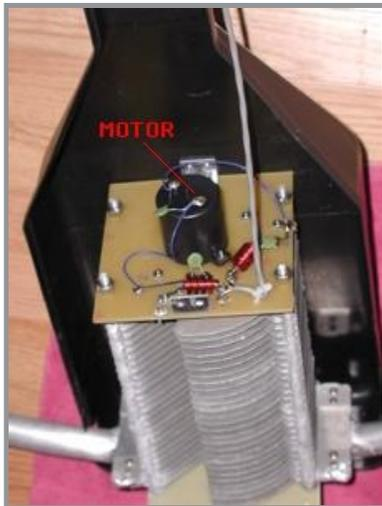
I guess you can file tonight's entry under, "I really didn't need any more problems, but..." The MFJ loop I've been using died again. Specifically, the small 1 RPM motor in the unit stopped working. This is the second replacement motor I've installed. The first, luckily, died while the unit was under warranty. And, true to MFJ's word, they sent me a free replacement quickly with no questions asked. This one was, now that the unit is out of warranty, \$40. {sigh}
