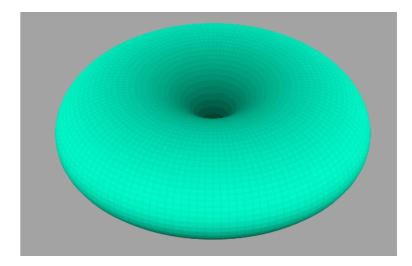
This is the radiation pattern of a quarter-wave vertical radiator with 30 radials just above good ground
